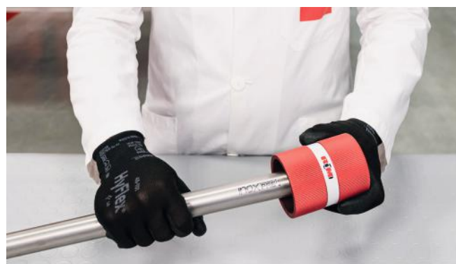
Figure 26 - Deburring the pipe
