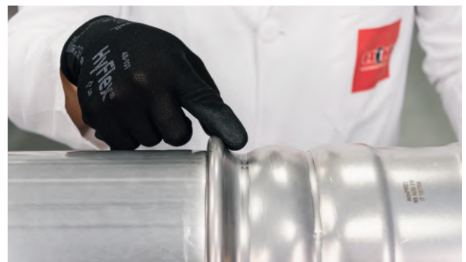
Figure 36 – Visual inspection of oversized pressing
