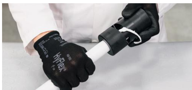
Figure 29 - Stripping (steelPRES PP coated)
